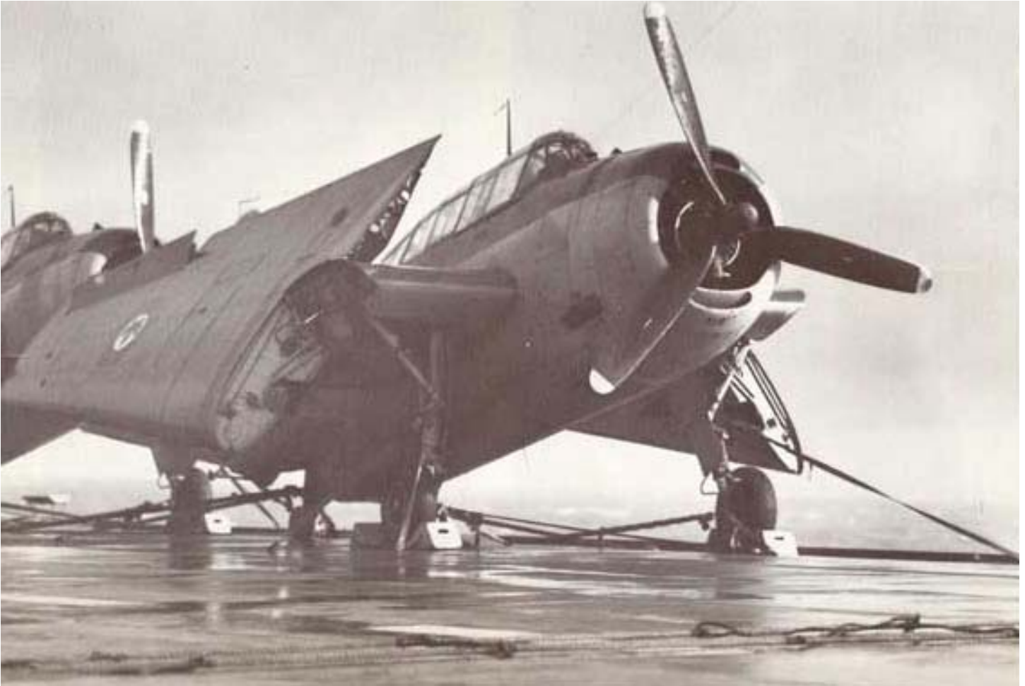
HP1. A TBM aboard aircraft carrier in 1945, photograph by United States Navy. Note wings in folded position. Original photo located in Still Picture Branch, (NNSP) records, Department of the Navy, Record Group 80, (RG80), National Archives of the United State, Washington, D.C.
